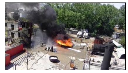
A scene from the recent testing LASTFIRE testing programme aimed at assessing the performance of new foam formulations – Fluorine Free and C6 fluorosurfactant based – for bund spill fire application
